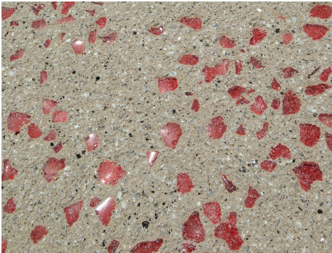
Proposed exposed aggregate using recycled glass.
